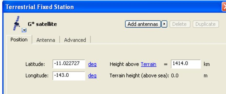
Figure 7.—Setting the position of a Globalstar satellite.
